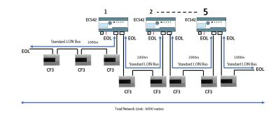
**Note:** Max 5 modules is permitted per LON bus network. EOL =  $120\Omega$
