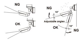
Keep the detection window straight and the adjusting part at the bottom
